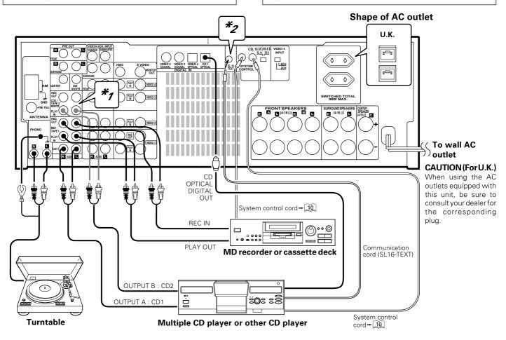
\*2 Note on the SL-16 TEXT jack (provided except for some destination areas): When using a KENWOOD CD player equipped with the SL-16 TEXT jack, connect it to this unit using the communication cord provided with the CD player. This makes it possible to display the disc and track titles on the remote control unit (provided with this unit). Do not forget to set the SL-16 / XS-8 switches of the CD player and this unit to SL-16.
